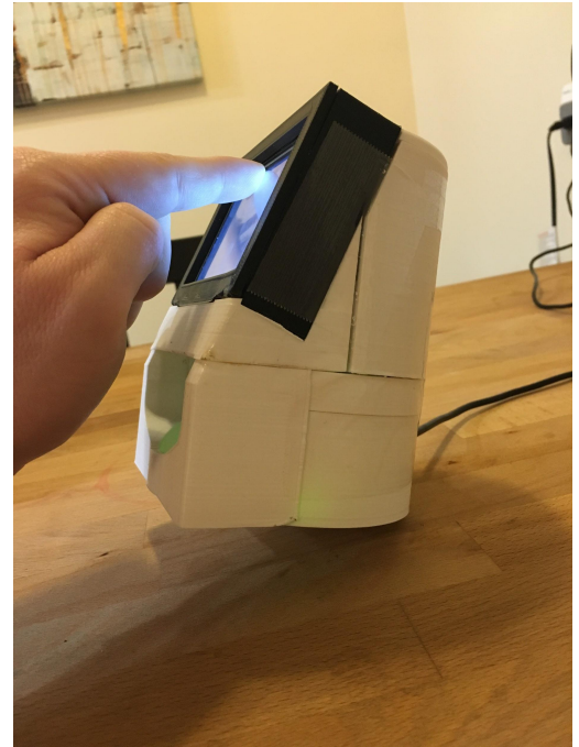
Device tipping when pressed.
